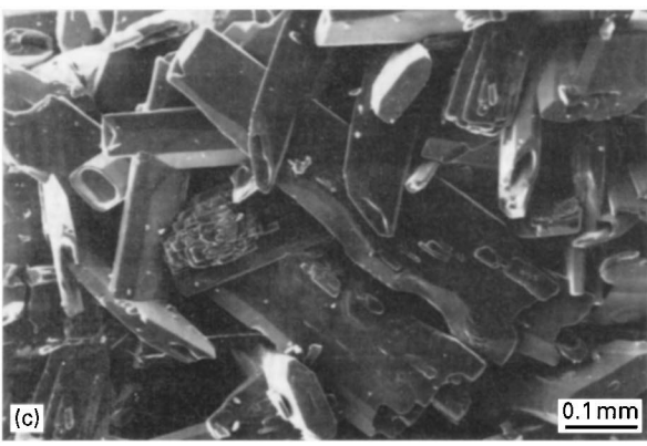
Figure 5 PSB tablets obtained after heating in chlorine for separated oxides disposition at 950 °C, (a,b) 4 h, (c) 24 h.
